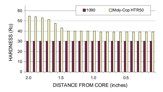
The higher hardness rods reduce mill consumption significantly. Moly-Cop HTR50 mill trials have shown consumption decreases of approximately 20% - 25% over 1090 rods.
