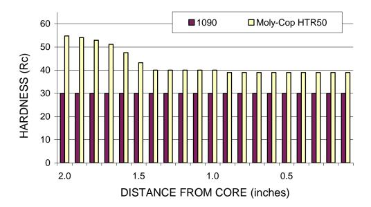
The higher hardness rods reduce mill consumption significantly. Moly-Cop HTR50 mill trials have shown consumption decreases of approximately 20% - 25% over 1090 rods.
